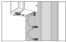
Protective bonding circuit - Double point connection
