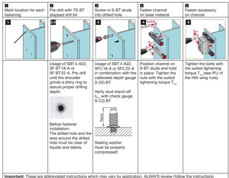
Important: These are abbreviated instructions which may vary by application. ALWAYS review/follow the instructions for use (IFU) accompanying the product. In case of a drill through hole, rework of the coating on the back side of the plate/profile may be needed.
