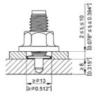
Fastened material hole ∅ ≥ 13mm (0.51")
