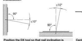
Position the DX tool so that nail inclination is limited to max. 10° from perpendicular to surface valley.
