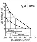
① Fastener: X-CRM8-\_\_-12 FP10 / Tool type: DX 76 (impact)
