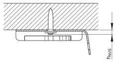
$h_{NVS, min} = 3 mm$  $h_{NVS, max} = 7 mm$  Admissible fastener stand-off X-MW ALH 22 (X-ALH 22)
