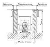
$t_{\text{bearing bar}}$  Bearing bar thickness  $w_{\text{clear bar spacing}}$  Clear bar spacing
