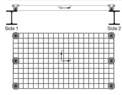
Grating element: X-FCS-R-4-25 Saddles connected to bearing bar: 4 Fastener: S-BT-GR M8/7 SN 6 Base material: S355 Base material thickness: t<sub>II</sub> = 6 mm
