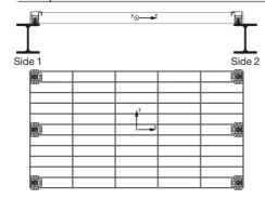
Grating element: X-FCS-R-3-25 Saddles connected to bearing bar: 2 Fastener: X-BT M8-15-6 SN 12 R Base material: S235
