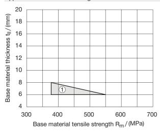
① X-R 14 P8 with DX 6 F8, X-R 14 P8 with DX 5 F8
