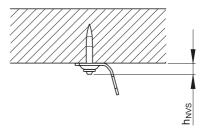
$h_{NVS, min} = 6 \text{ mm}$  $h_{NVS, max} = 11 \text{ mm}$
