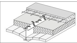
Typical application of X-HVB shear connector with jack arch system (without steel deck), e.g. rehabilitation project. "Duckwalk"
