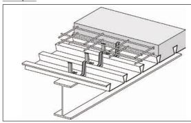
Typical application of X-HVB shear connector with steel deck, e.g. new construction.
