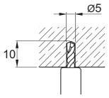
Pre-drilling with Hilti drill bit **TX-C-5/10B** until a ring on the concrete surface is visible.
