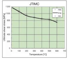
At 600°C, the CR500 material has 64% of its 20°C shear strength left. By comparison, standard fasteners have only 12% and structural steel only about 26%. The excellent fire resistance of the CR500 material alone justifies its use for some applications.
