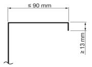
Fastening to U-shape concrete inlays with a nominal thickness  $t_{II}$  of 3 mm.  $t_{II} = 3.0 \pm 0.3$  mm
