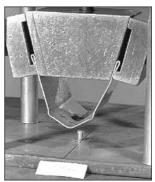
Pull-over test specimen at test start Sheet pull-over
