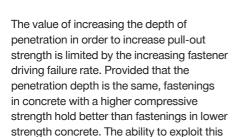
Pull-out strength and fastener driving failure rate both increase with increasing penetration depth. The optimum depth of penetration is taken as the depth at which the yield in terms of pull-out strength begins to decrease. This is within a range of 18–32 mm depending on the grade and age of the concrete as well as the strength of the fastener.
